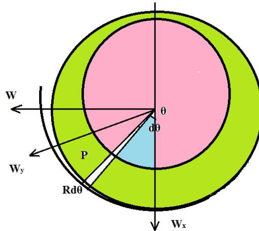
Figure3. Geometry for Components of Load Capacity
