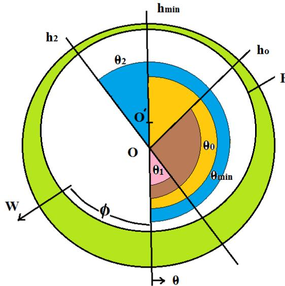
Figure 1. Geometry of Journal Bearing
