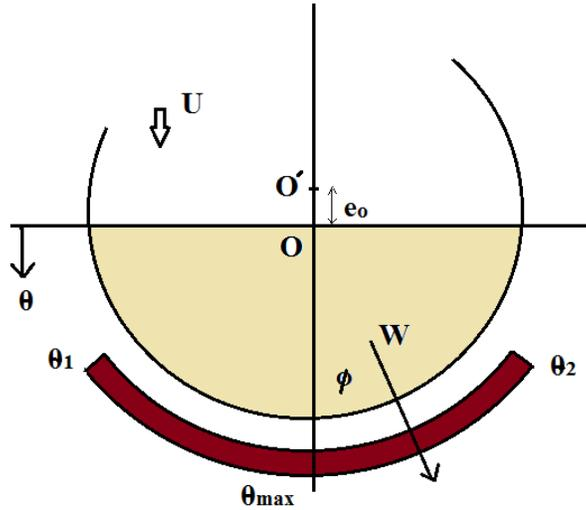
Figure2. Geometry of Fitted Bearing
